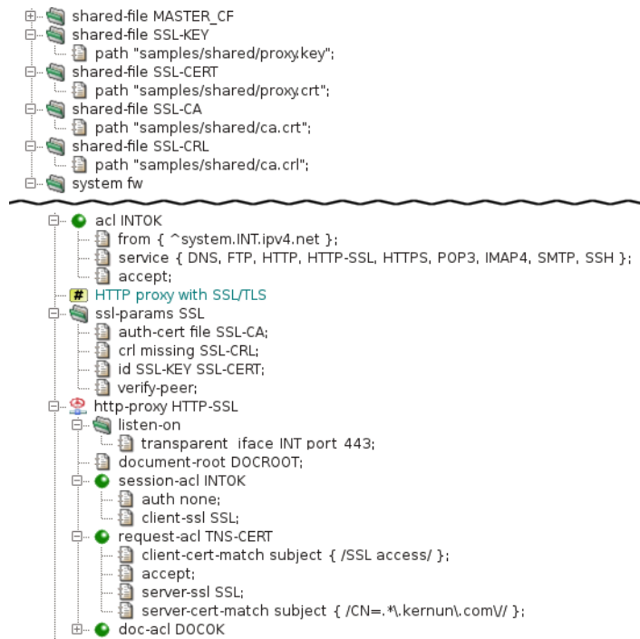
Figure 5.39: SSL/TLS security configuration
