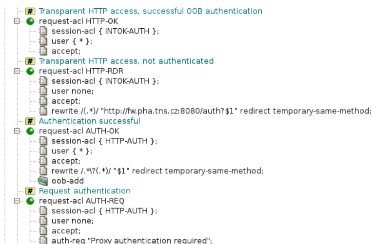
Figure 5.48: Transparent Kerberos authentication — request ACLs
