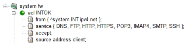
Figure 5.32: Transparency for servers ( source-address client )
